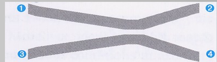
Fig. 2.3.7b Directional coupler with sliding, position-dependent coupling
